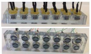
Figure 2. The microfluidic-WCL containing 14 ISE sensors interconnected by a sub-mm flow channel requiring only 100  $\mu$ L of sample solution.
